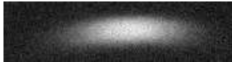
Figure 6.14: Fluorescence image taken of the atom cloud 100 ms after release from the MOT 10 mm above the 3 mm mirror. Again a slight curvature is seen, though less dominant than for the 10 mm mirror.
